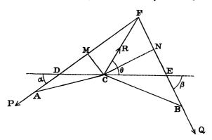
given forces acting at A and B, and R the pressure on C.
